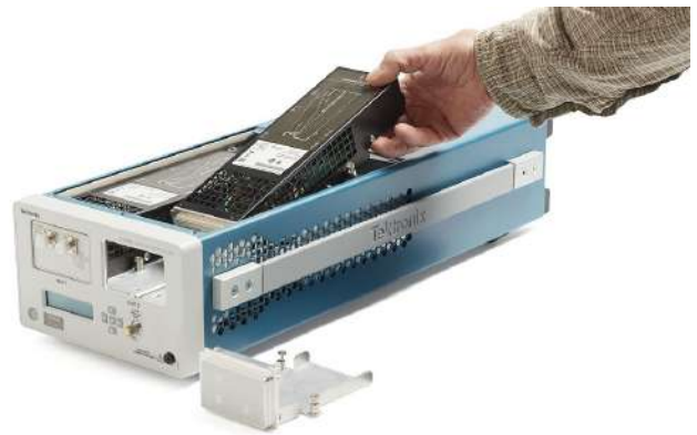
Plugging TSO8C18 module into TSO820 mainframe.
